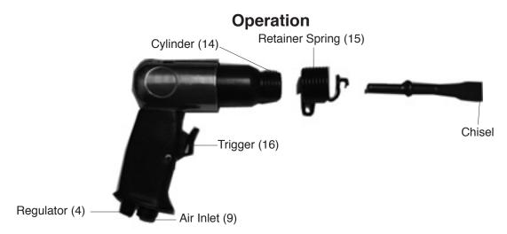
Examine your chisels/bits before using them. If a chisel is dull or cracked do not use it. Replace worn or broken chisels with approved replacement chisels/bits from Harbor Freight Tools.
